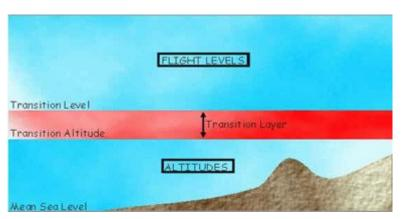
Figure 3.1: Illustration of Transition Level, Transition Layer and Transition Altittude.
