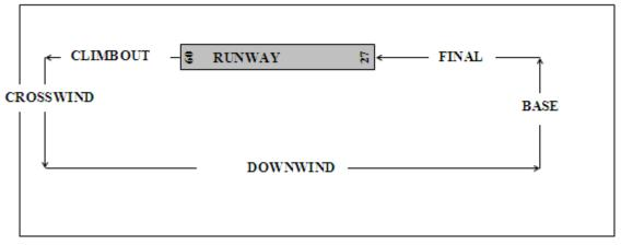
Figure 5.1: A typical left-hand circuit.
