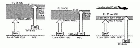
Figure 3.2: Illustration of Minimum Usable Flight Levels.
